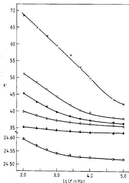
**Figure 15.** Frequency dependency of the dielectric constant ( $\epsilon'$ ) for different fixed temperatures (K): (●) 77, (▲) 530, (△) 580, (●) 625, (○) 650, (×) 680 [24].
