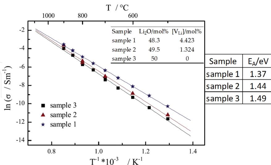
**Figure 12.** Arrhenius representation of the electrical conductivity of single-crystalline LN samples with different lithium contents, in the temperature range between 500 and 900°C.  $[V_{Li}]$  represents the mol% of lithium vacancies, calculated through the lithium vacancy model (Eq. (1)). The activation energies ( $E_A$ ) for the different samples are also indicated (adapted with permission from [6]).
