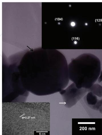
**Figure 9.** TEM bright-field micrograph of the LN particles prepared by the reactive molten salt synthesis (RMSS). Inset on the top right: selected area electron diffraction pattern of the area marked by the black arrow. Inset on the left bottom: high-resolution micrograph of the area marked by the white arrow [10].
