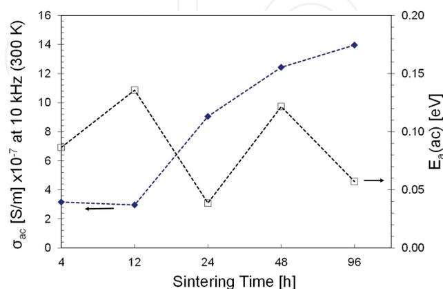
**Figure 29.** Ac conductivity ( $\sigma_{\text{dc}}$ ) and activation energy ( $E_a(\text{ac})$ ) of the samples sintered at  $450^\circ\text{C}$  for 4, 12, 24, 48, and 96 h, at 10 kHz and room temperature (300 K).
