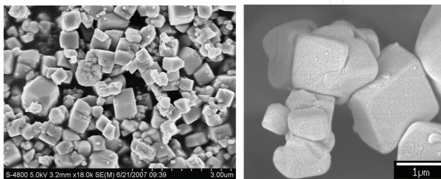
**Figure 8.** At left: SEM micrograph of polycrystalline LN prepared by a low-temperature hydrothermal route [21]. At right: SEM micrograph of polycrystalline LN prepared by the reactive molten salt synthesis (RMSS) process [10].
