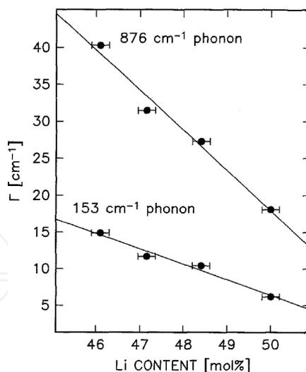
**Figure 6.** Full width at half maximum of the Raman lines at the wavenumbers 153 and 876  $\text{cm}^{-1}$ . The dots are experimental values obtained for samples with different lithium contents (mol%), at room temperature, and the lines are the linear least-squares fits [19].
