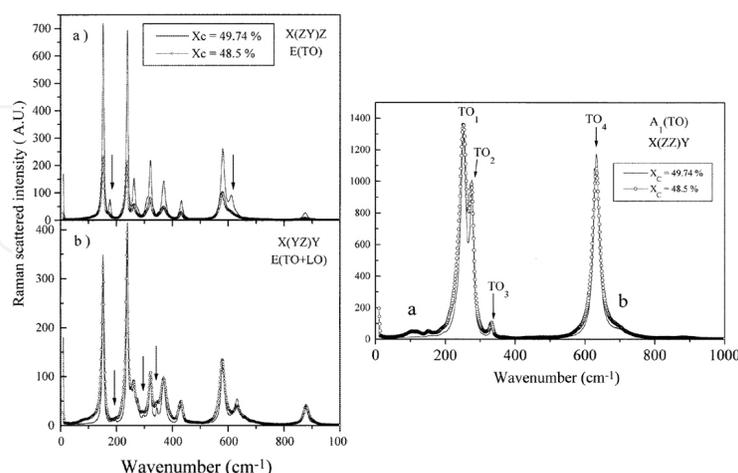
**Figure 7.** At left: Raman spectra of two LN crystals with composition  $x_c = 49.7\%$  (nearly stoichiometric) and  $x_c = 48.5\%$  (congruent), exhibiting the E(TO) and E(LO) vibrational modes. The arrows highlight lines that are more clearly visible in the nearly stoichiometric composition. At right: the configuration X(ZZ)Y allows the detection of the  $A_1$ (TO) phonons [18].
