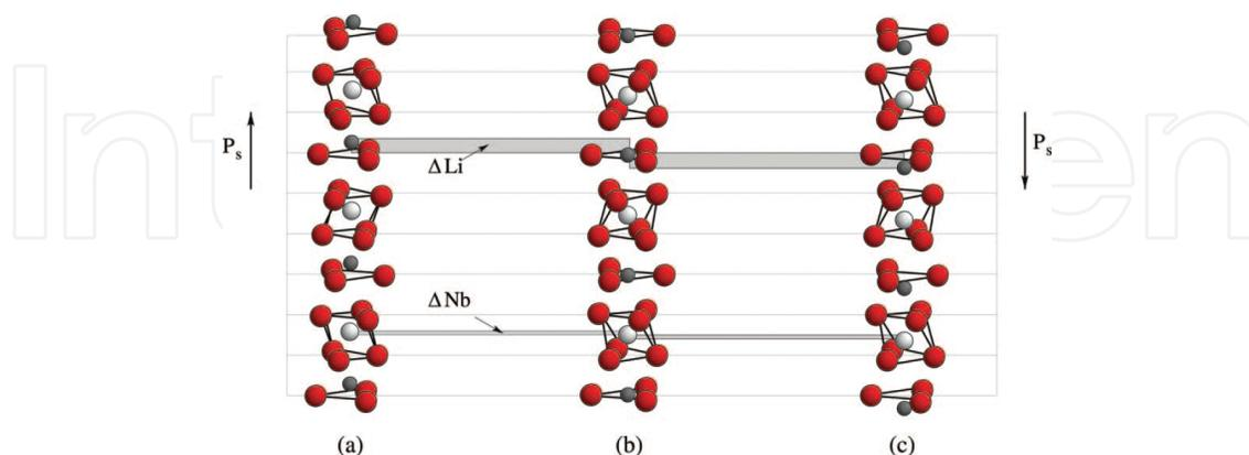
**Figure 2.** (a) and (c) Atomic model of the LN ferroelectric phase. (b) Atomic model of the LN paraelectric phase.  $\Delta\text{Li}$  indicates the displacement along the c-axis of the  $\text{Li}^+$  cations, represented as black spheres, while  $\Delta\text{Nb}$  indicates the displacement along the c-axis of the  $\text{Nb}^{5+}$  cations. Both displacements are represented relatively to the center of the oxygen (red spheres) planes [14].
