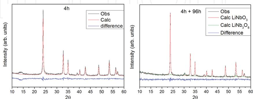
**Figure 23.** The Rietveld fits of the XRD patterns for the powder HT at 450°C, containing only the LN crystalline phase and the sample sintered for 96 h, containing both LN and  $\text{LiNb}_3\text{O}_8$ .
