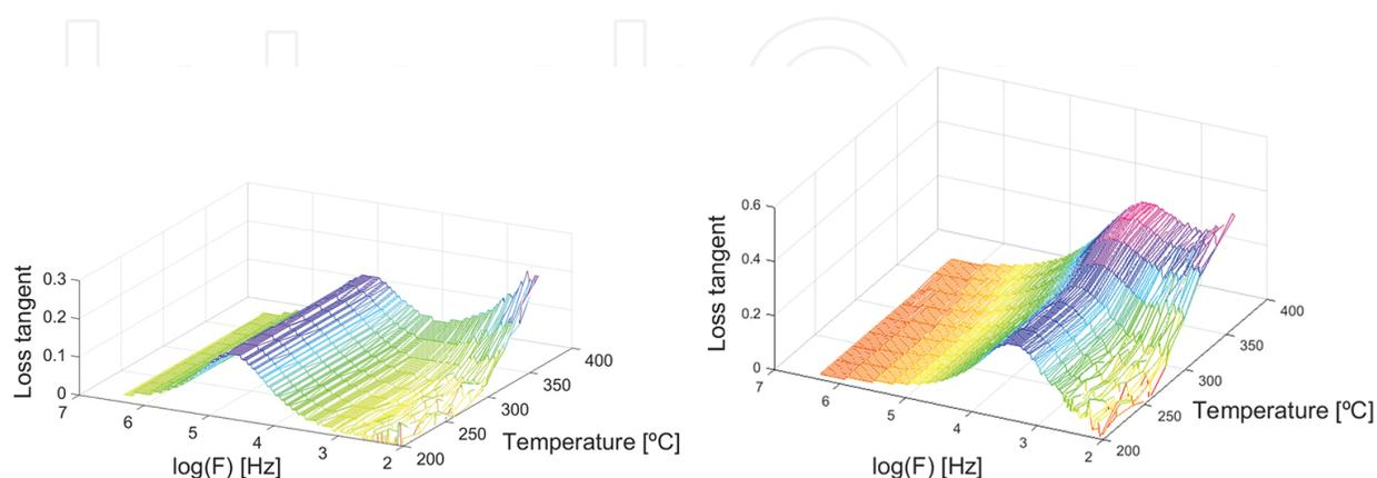
**Figure 31.** At left: dependency of the loss tangent with the temperature and frequency for the sample sintered at 450°C for 24 h. At right: dependency of the loss tangent with the temperature and frequency for the sample sintered at 450°C for 96 h.
