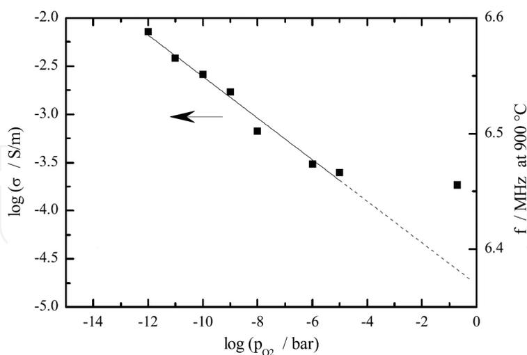
**Figure 10.** Dependence of a LN stoichiometric sample (sample 3 of **Figure 12**) total electrical conductivity with the oxygen partial pressure  $p_{O_2}$ , at 1173 K (900°C). The solid line is the linear fit of the experimental values, while the dotted line is the extrapolation [6].
