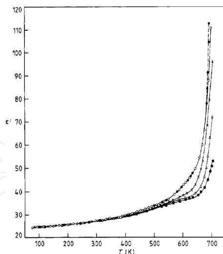
**Figure 16.** Temperature dependency of the dielectric constant ( $\epsilon'$ ) for different fixed frequencies (kHz): ( $\circ$ ) 0.1, ( $\times$ ) 1, ( $\Delta$ ) 10, ( $\blacksquare$ ) 100, ( $\bullet$ ) Sample with half of the thickness, keeping the same area [24].
