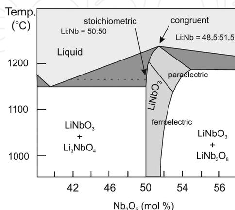
**Figure 1.** Phase diagram of the Li<sub>2</sub>O-Nb<sub>2</sub>O<sub>5</sub> binary system [3].
