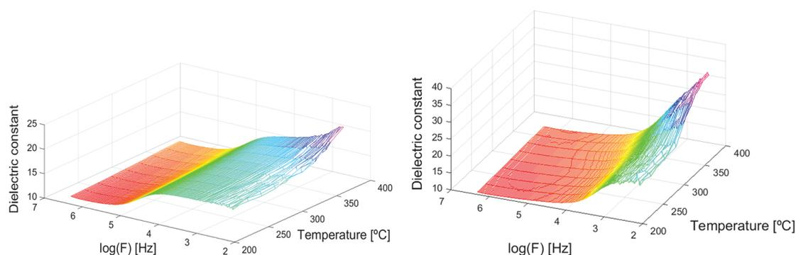
**Figure 30.** At left: dependency of the dielectric constant with the temperature and frequency for the sample sintered at 450°C for 24 h. At right: dependency of the dielectric constant with the temperature and frequency for the sample sintered at 450°C for 96 h.
