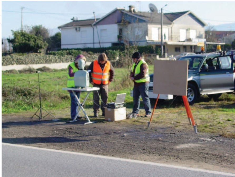
Figure 4. Measuring systems for SPB tests: microphone and HATS.
