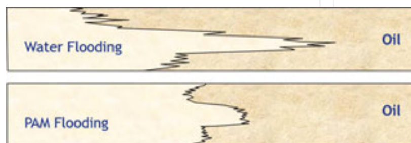
Figure 1. Water breakthrough can be delayed and sweep efficiency improved by increasing the viscosity of the injected fluid with polyacrylamide polymers (PAM) (modified with permission from Sorbie [11]).
