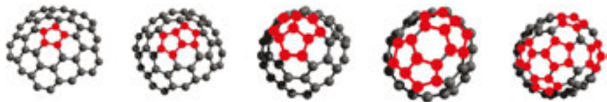
Figure 2. Conical nanostructures with different numbers of pentagonal defects in the tip.
