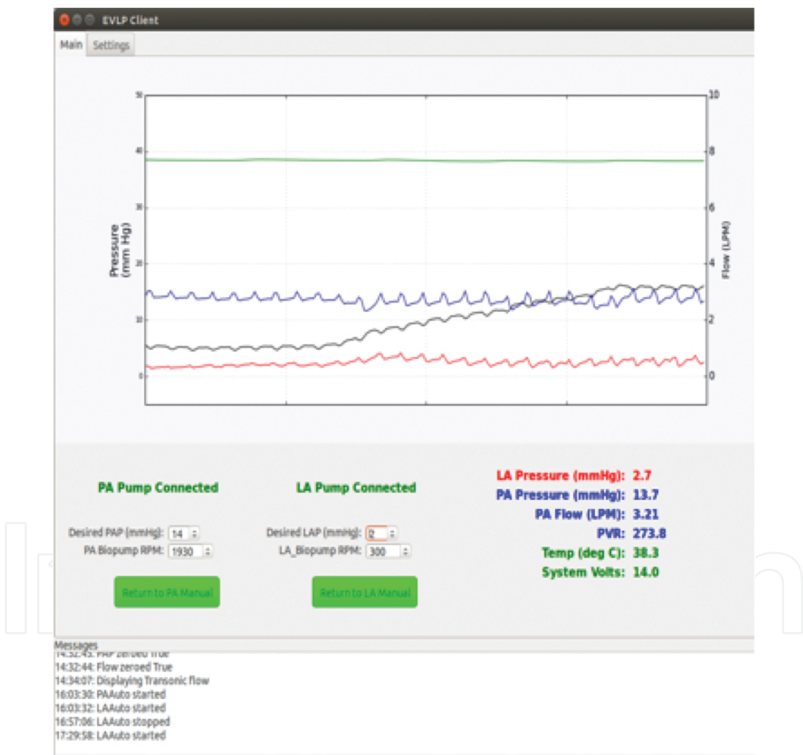
Figure 4. Microcontroller interface for the EVLP circuit parameters.
