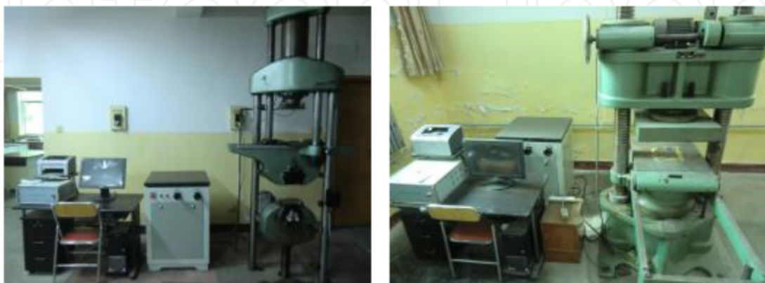
Figure 2. 60 t Universal Bending Test Machine and 200 t Compression Testing Machine.
