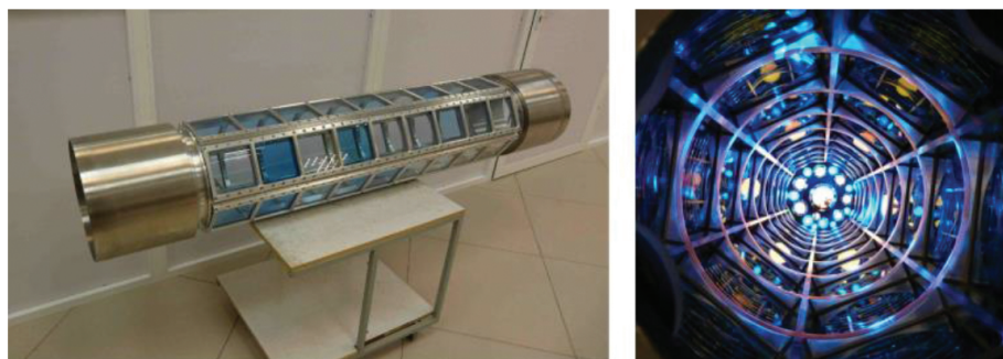
Figure 9. (a) Laser cell of the XeF(C-A) amplifier. (b) Inside view of the laser cell with the mirror unit.
