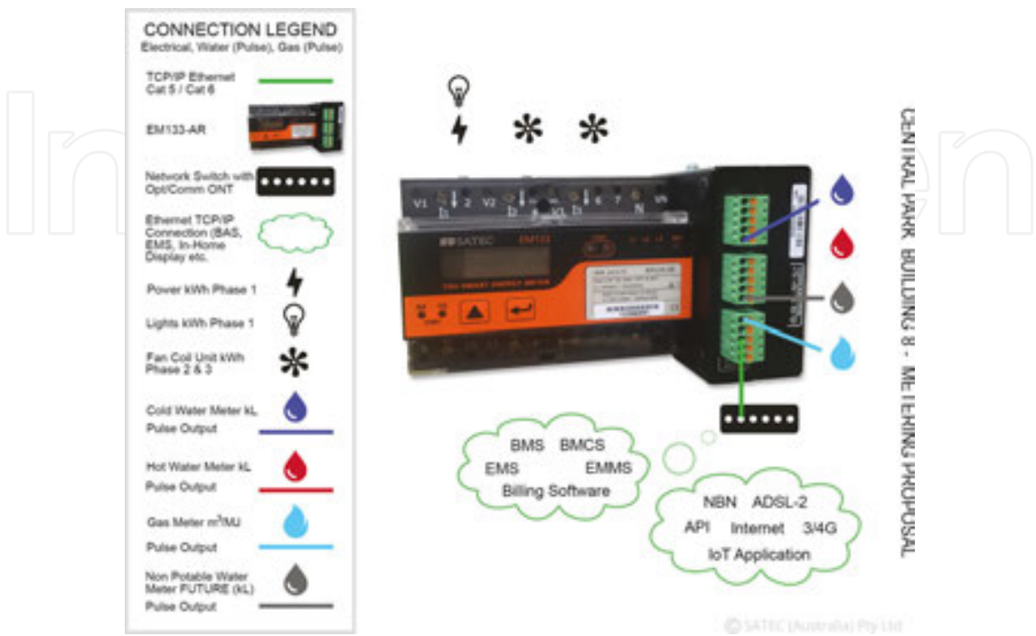
Figure 11. Central Park—Proposed Building 8 Solutions (Mechanical, Electrical, Hydraulic Services).
