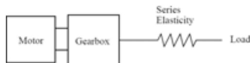
Figure 1. Series elastic actuator schematic (Williamson, 1995).
