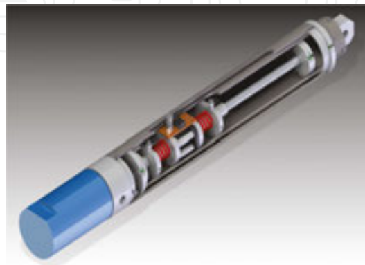
Figure 12. Actuator final design with internal components.
