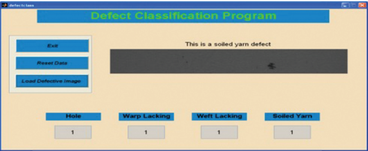
Figure 20. Classification of soiled yarn defect.
