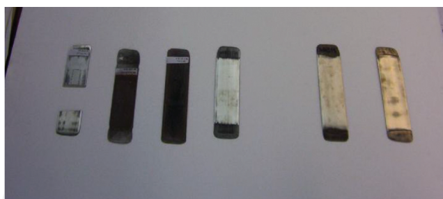
Figure 15. Monolithic \gamma -U7Mo/Zry-4 miniplates used along the different development stages. The three at the right extreme are in an intermediate step of surface oxide removal.
