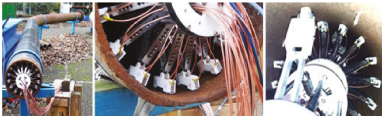
Figure 29. LRU collar for pipeline monitoring.
