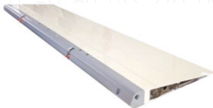
Figure 25. Photograph of the aileron prototype.
