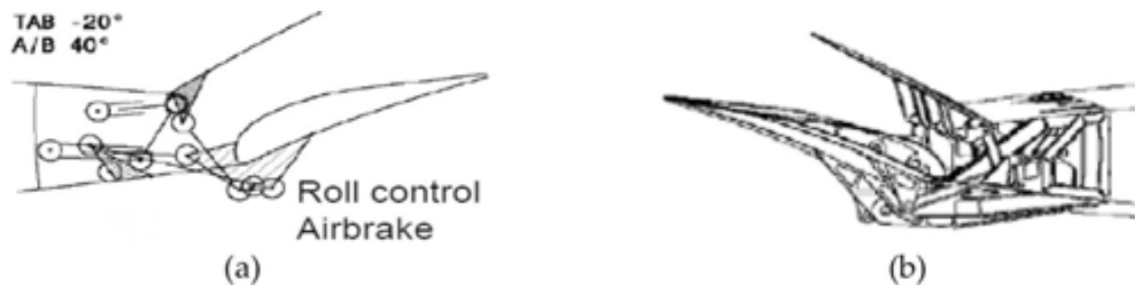
Figure 8. A350 XWB (Extra-Wing Body) with A/B and tab deflection for roll control maneuver [6].
