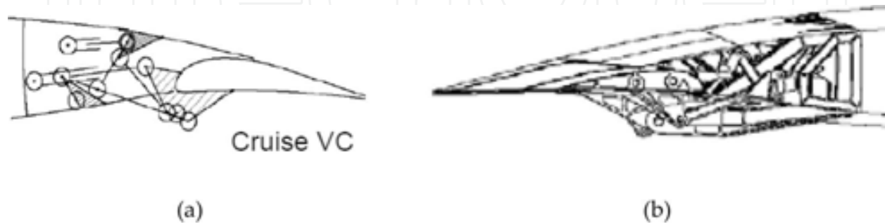
Figure 7. A350 XWB (Extra-Wing Body) flap in cruise condition [6].
