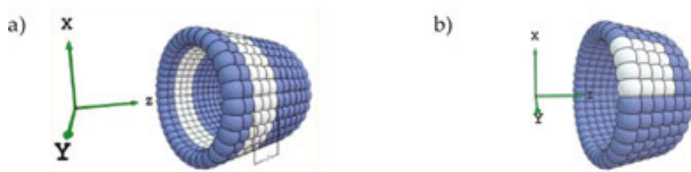
Figure 7. Cluster models of TiO 2 (001) NTs: (a) ring fragment and (b) arc segment of ring.
