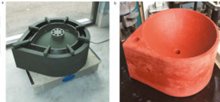
Figure 15. (a) Printed form mounted (form for casting upside down) and (b) designer sink made from concrete.
