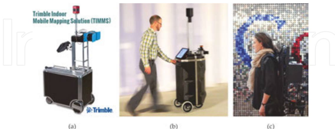
Figure 11. Indoor mapping systems: TIMMS (a), iMMS (b) and CARTOGRAPHER (c). Images courtesy of Trimble, SmartGeometrics and Google, respectively.
