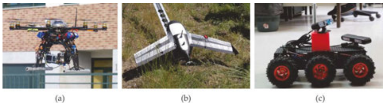
Figure 7. Unmanned vehicles employed in forensic science. Multirotor (a); fixed-wing (b) and ground vehicles (c).
