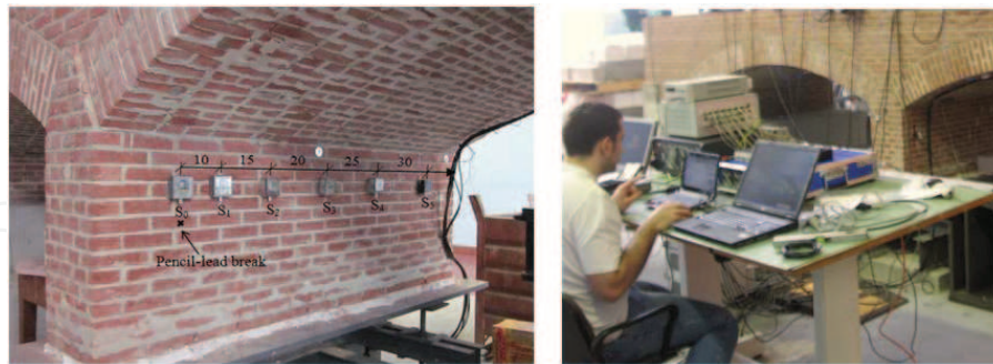
Figure 6. Wave velocity test: (left) the sketch of the pencil-lead break point and the sensor distribution and (right) scenario of the velocity test.
