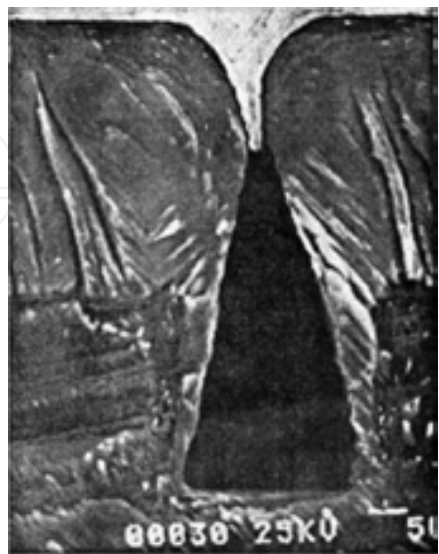
Figure 5. A vapor-deposited micro-grooved heat pipe [17].
