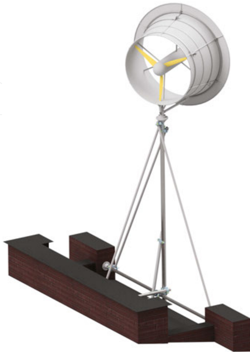
Figure 6. Roof-mounted SWT equipped with the diffuser.
