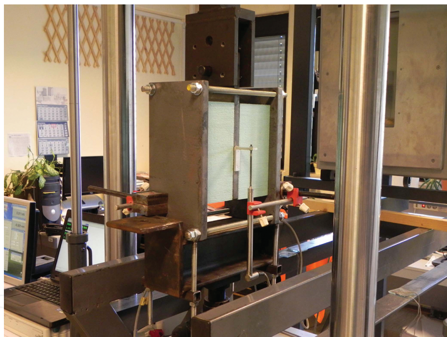
Figure 5. The XPS shear test setup.
