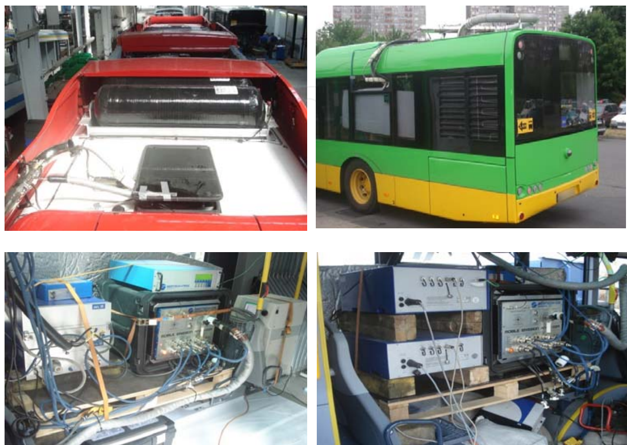
Figure 5. City buses prepared for the tests (left - CNG -fueled vehicle).
