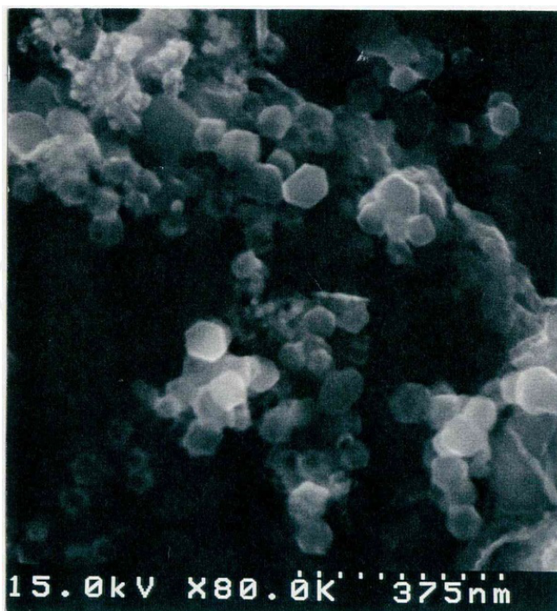
Figure 8. SEM micrograph of W-Ti sample for run No. 7, heat treated at 850°C for 2 h.
