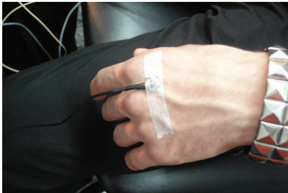
Figure 6. Example of the reference disc electrode placement.
