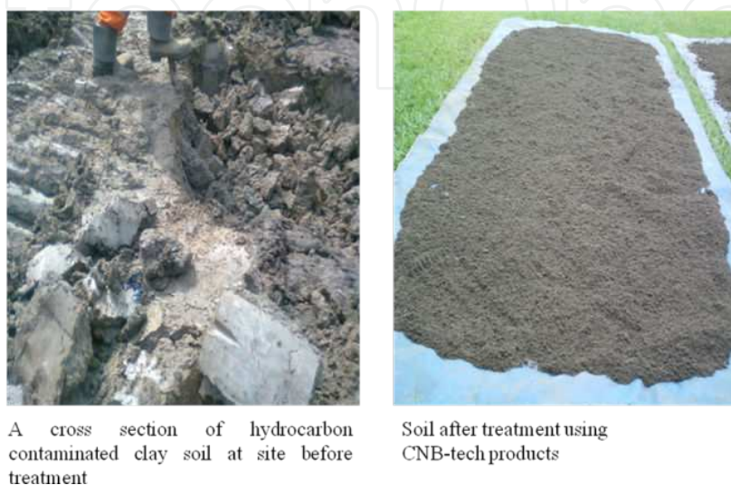
Figure 8. Appearance of the crude-oil-impacted clay soil before and after CNB-Tech treatment
