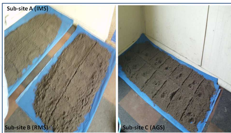
Figure 5. The three different sample bulks showing grid template of 12 cells created on each sample, from which samples were collected for physicochemical analyses
