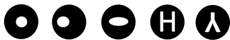
Figure 7. Cross Sections of Sheath Core Bicomponent Fibers
