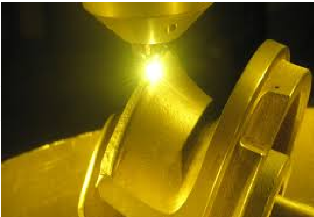
Figure 8. Fabrication of impeller pump using LENS™ [40].
