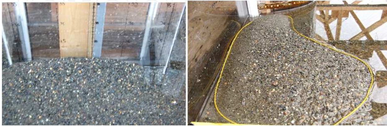
Figure 5. Scour pattern with nonuniform sand from Case 1
