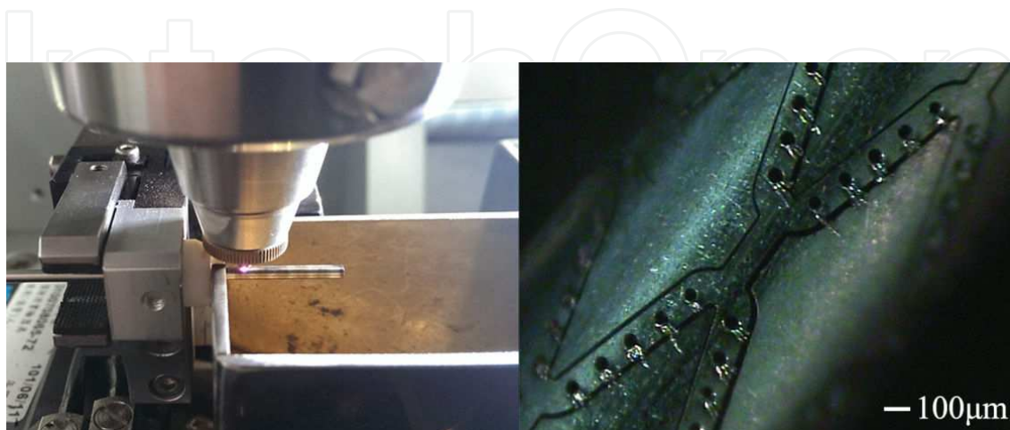
Figure 6. Stent design pattern cut onto a seamless hypotube by laser.
