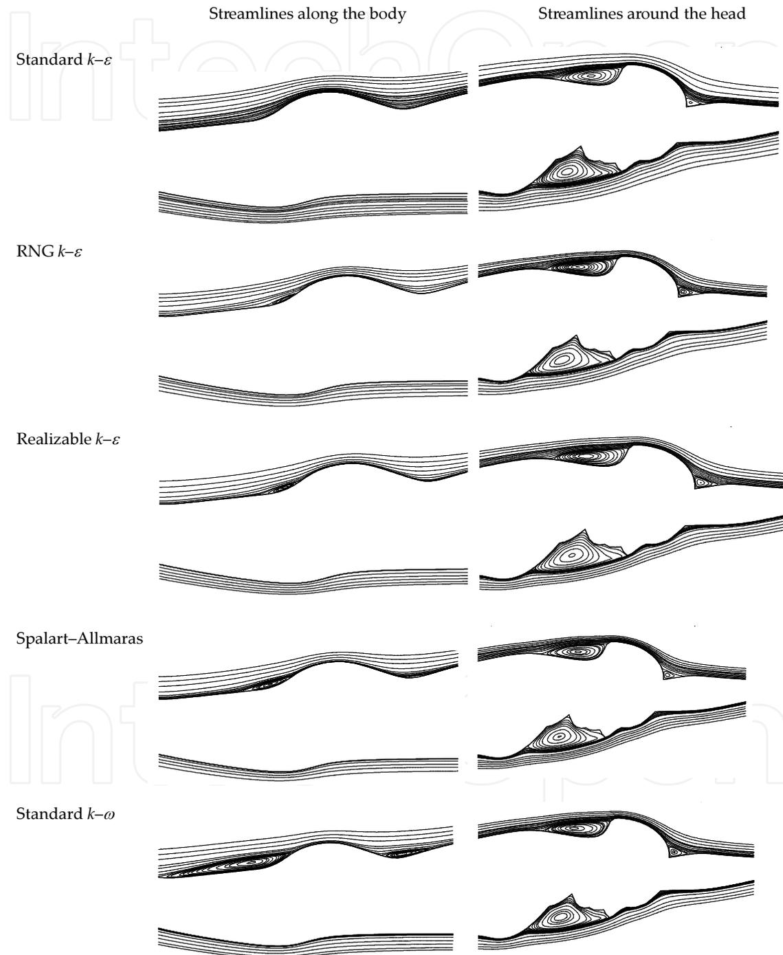
Figure 2. Streamline patterns around the swimmer's body. Swimmer's speed:  $U_0 = 2.2$  m/s.
