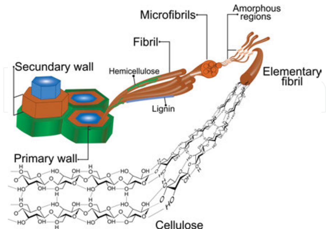
**Figure 1.** Hierarchical structure of cellulose extracted from plants.
