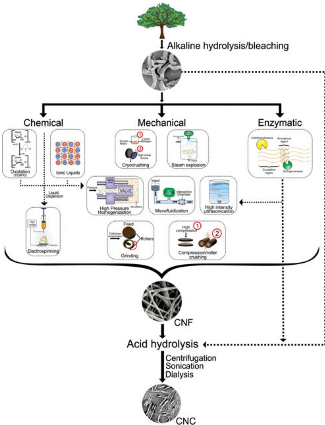
Figure 2. Conventional treatments to obtain cellulose nanoparticles.
