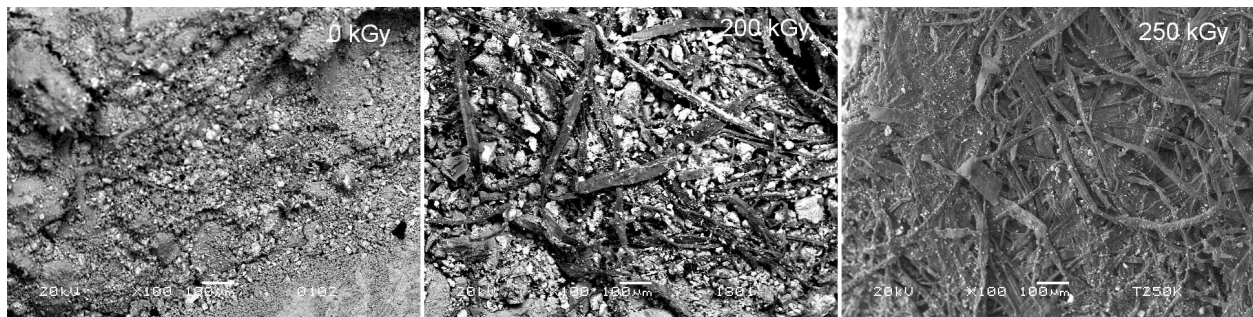
Figure 5. SEM images of gamma-irradiated concrete with tire rubber fibers
