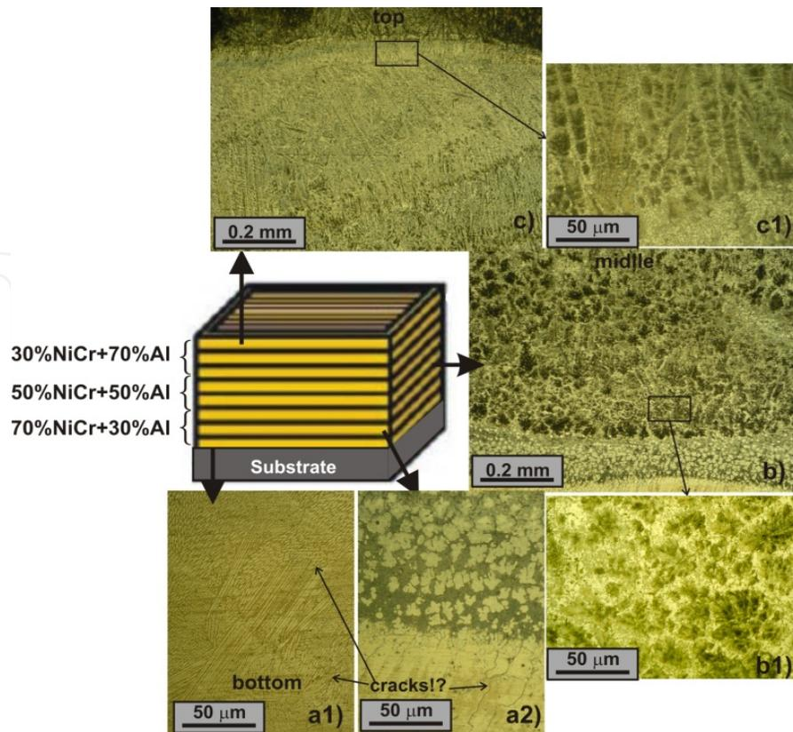
**Figure 3.** OM micrographs showing the typical microstructures of 3D laser clad coating of NiCr–Al multilayer system: (a) bottom layers ~2–4 mm from substrate; (b) middle layers ~4–6 mm from substrate; (c) top layers ~6–8 mm from substrate.
