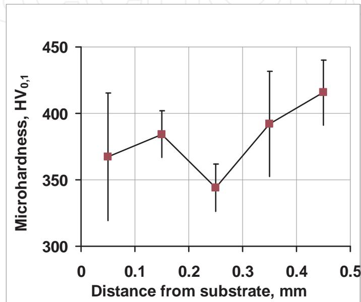
**Figure 10.** Microhardness distributions of the Ni85Al15 after the multilayer DMD.
