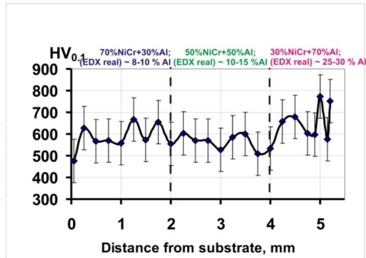
Figure 4. Microhardness distributions of NiCr–Al FG multilayer system.
