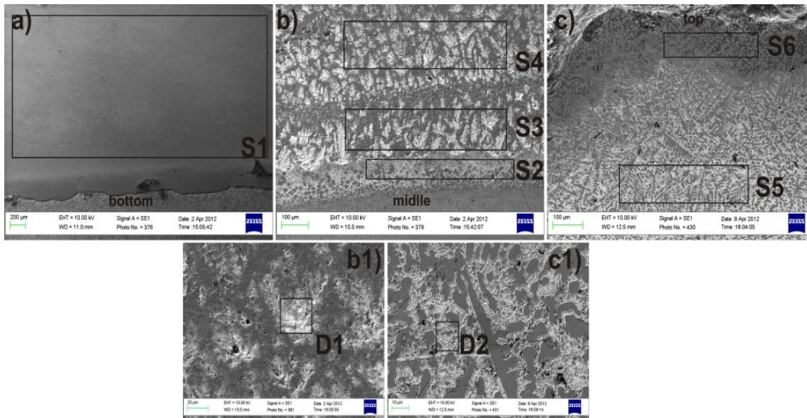
**Figure 6.** SEM micrographs showing typical solidification microstructures of the bottom (a), middle (b), and top (c) deposited layers with places of the EDS analysis of NiCr–Al multilayer gradient (see Table 1).
