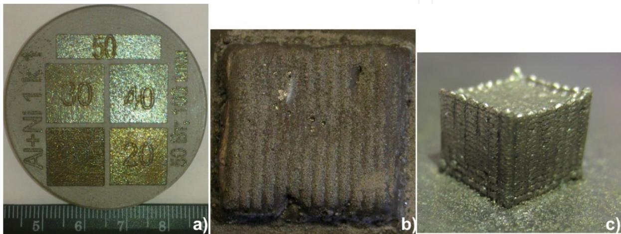
**Figure 2.** Appearance of the SLM and DMD processes: (a) SLM in Al + Ni = 1:1 system, three layers, hatch distance 0.1 mm; (b) FGS in Ni–Al after DMD; (c) DMD of cube (5 mm<sup>3</sup>) from the Ni85Al15 powder.
