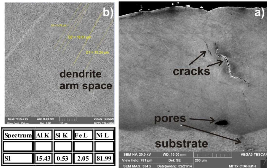
Figure 12. SEM micrographs showing typical solidification microstructures of the laser deposited layers with the laser scanning speed of 600 mm/min, 250 W, and 9 g/min. Step between the layers was 200 μm, and EDS analysis date (table) from whole image square.
