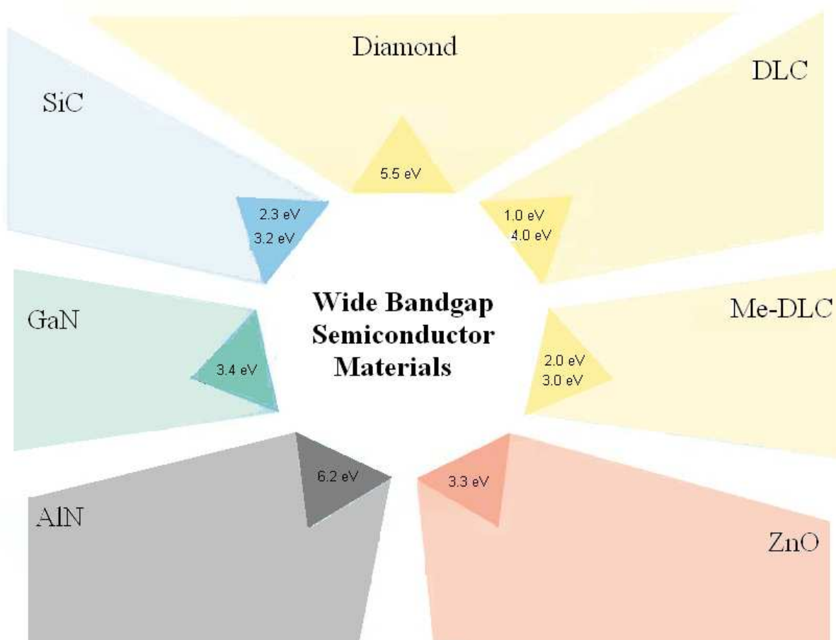
Figure 1. Wide bandgap semiconductor materials with potential for use in microsystem technology
