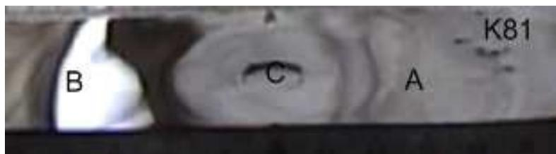
**Figure 19.** The start of the movement associated with the liquid layer on the surface of the gelatin block 81. A - bound fluid layer; B - bound (shaft) move "free" liquid; C - free gelatin surface.
