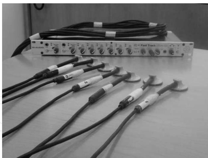
Figure 2. Multi-channel equipment for computerised respiratory sound analysis.
