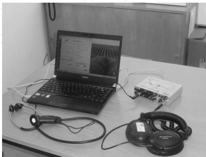
Figure 1. Single-channel equipment for computerised respiratory sound analysis.
