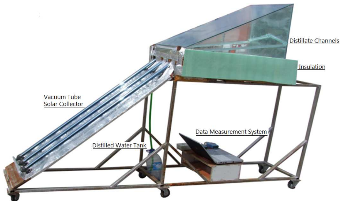
Figure 19. Vacuum tube collector assisted solar distillation system [34]
