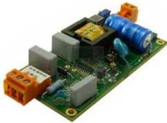
Figure 10. LEDs powered by a Flyback converter.
