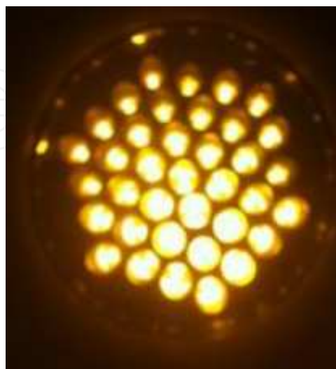
Figure 4. Arrangement of high brightness LEDs that emit amber light.
