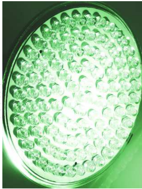
Figure 3. Arrangement of high brightness LEDs that emit green light.
