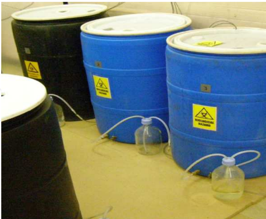
Figure 20. Disintegration barrels used to assess plastic fragmentation in an aerobic composting environment according to AS ISO
