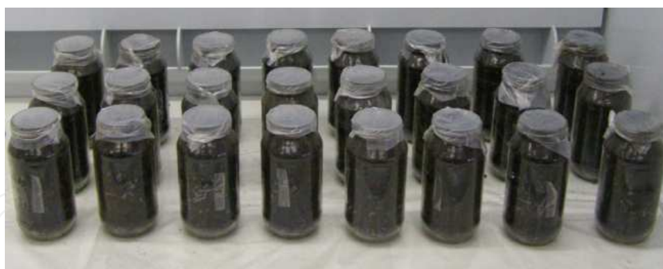
Figure 22. Photo of an earthworm ecotoxicity test setup ecotoxicity testing mung
