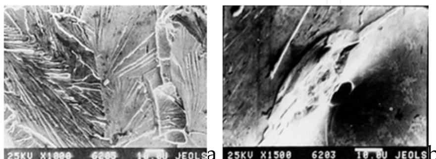
Figure 15. Fracture surfaces of molybdenum: (a) mixed fracture (double EBM run); (b) void, formed after breakaway of carbide (EBM+VAM).
