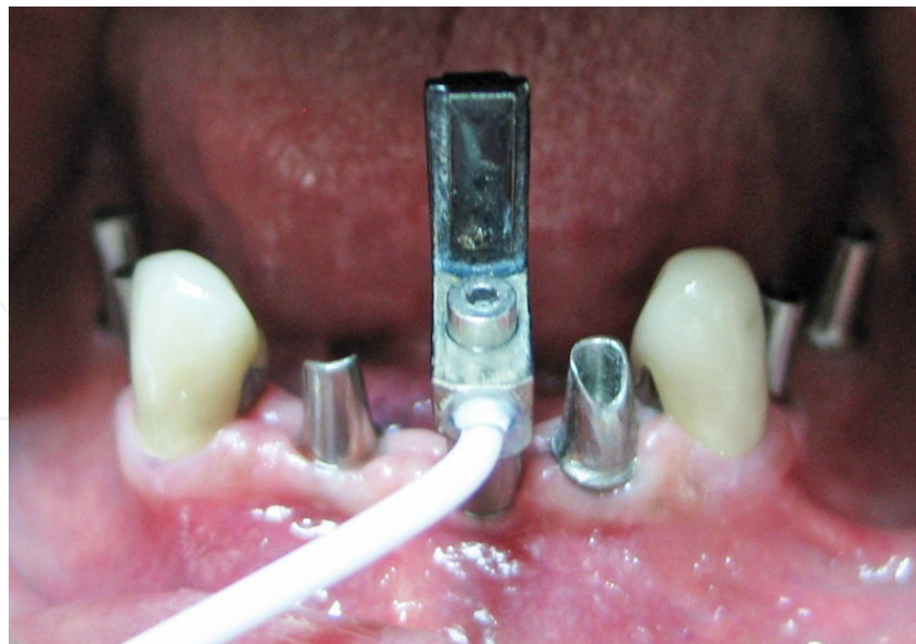
Figure 15. Transducer of Osstell instrument attached to implant for measurement.
