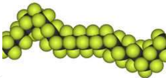
Figure 1. Typical interwined PTFE polymer. Due to strong intermolecular forces, the polymer chains are tangled. Due to its chemical inertness, PTFE cannot be cross-linked.
