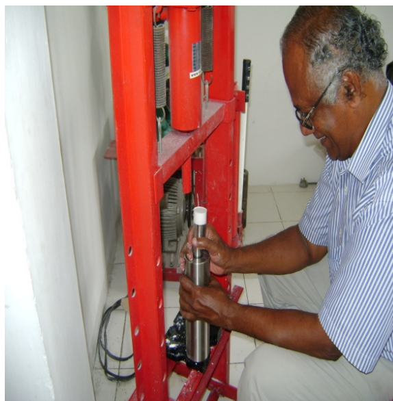
Figure 17. Mixture being cold pressed into pellet.
