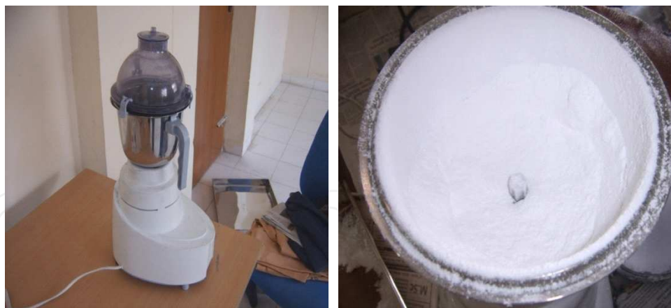
Figure 16. Ground PTFE powder being mixed with virgin PTFE powder.
