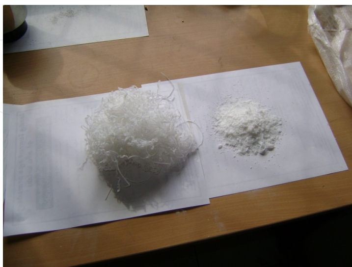
Figure 6. PTFE scrap before (left) and after gamma irradiation (right)
