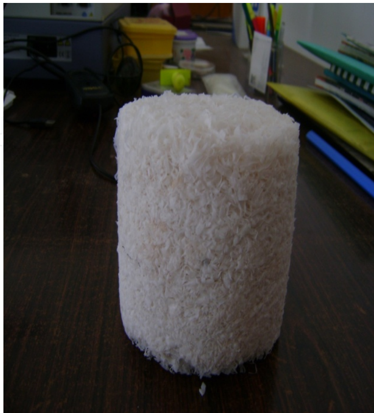
Figure 13. Shredded PTFE scrap after pre-heating treatment
