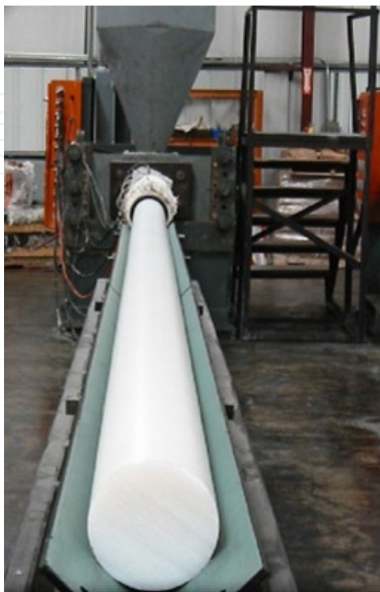
Figure 26. A typical ram extruder with 100% virgin extruded PTFE rod.
