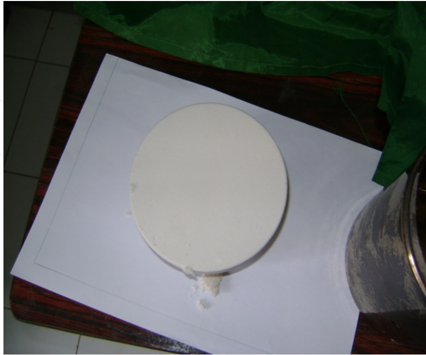
Figure 14. Pre-sintered scrap powder
