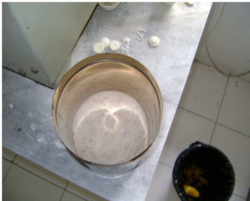
Figure 15. Ground scrap powder after pre-sintering
