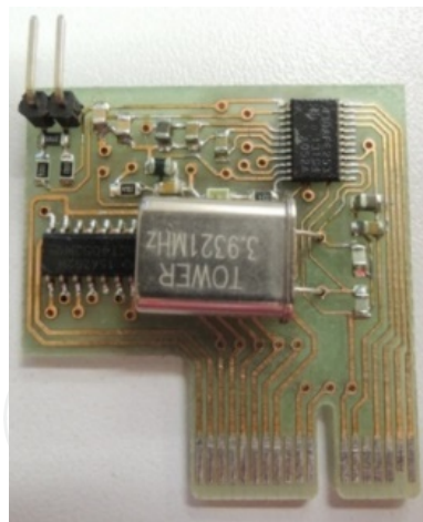
Figure 4. Prototype of the smart meter module [33].
