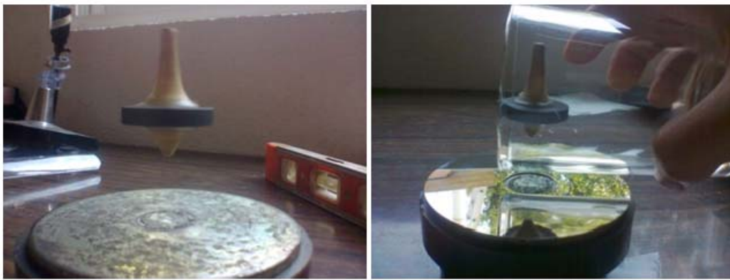
Figure 6. Magnetic levitation by fast rotating magnet.
