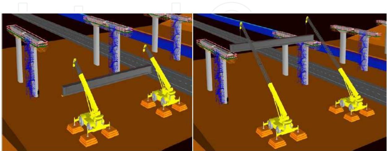
Figure 13. Prefabricated beams raised by two cranes.
