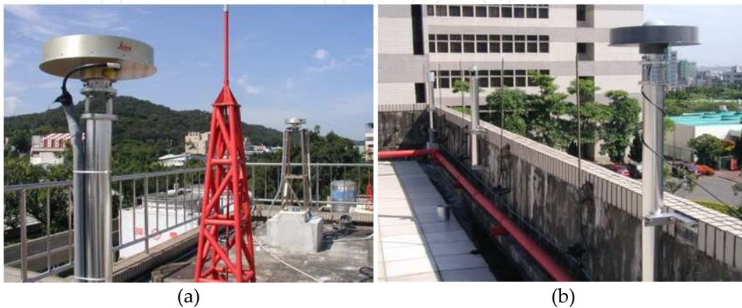
Figure 2. (a) Appearance of fixed stations; (b) Appearance of pillars of calibration base points [1]
