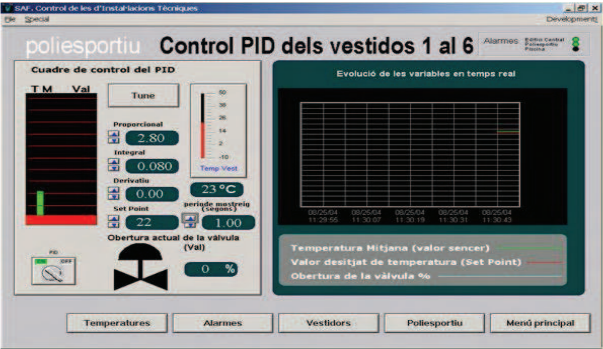
Fig. 5. An example of a Temperature feedback loop inside a SAF installation, and the ISA-PID control law used to close/open the regulation valve
