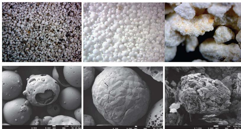
**Figure 11.** Examples of lightweight filler: cenospheres, bubble alumina and fireclay.
