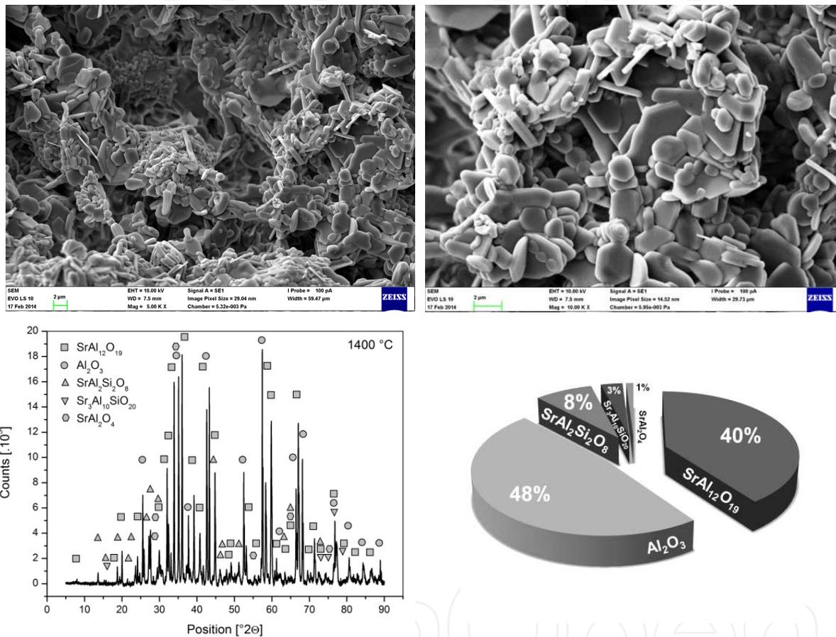
**Figure 8.** Electron microscopy image of refractory castable treated to the temperature of 1400°C.
