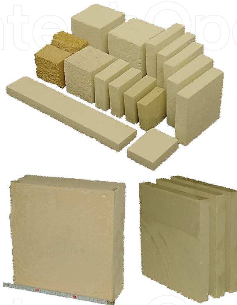
**Figure 21.** Examples of refractory foam prepared with calcium aluminate cement (a). Raw and fired block of ceramic foam (b).
