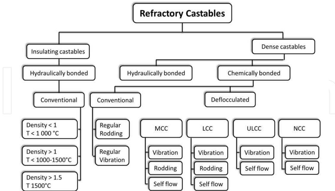
**Figure 2.** Types of Refractory Castables [455].
