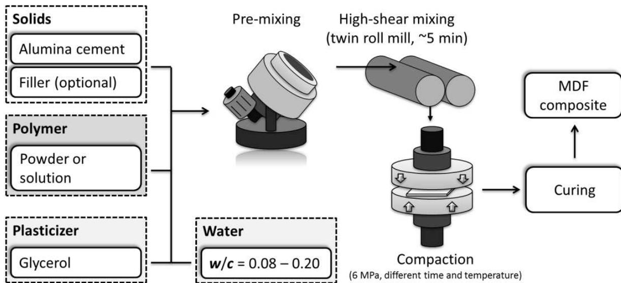
**Figure 27.** Typical stages of MDF manufacturing process [592].
