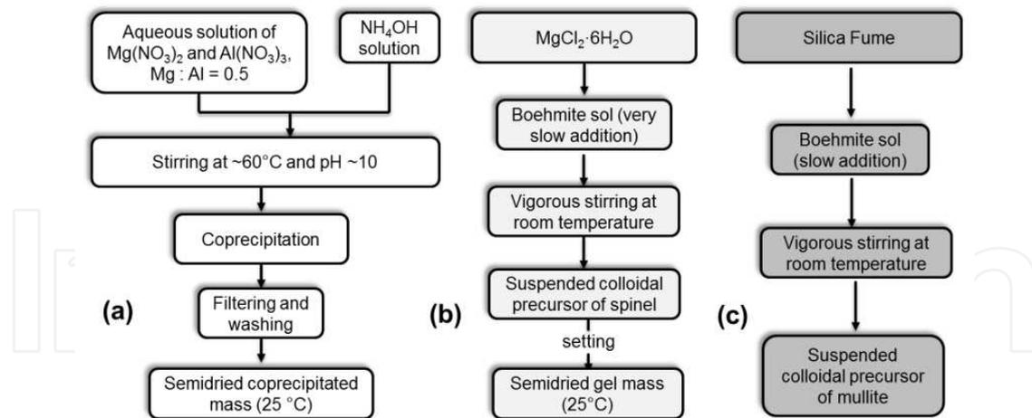
**Figure 3.** Preparation of co-precipitated spinel (a), sol-gel derived spinel (b) and mullite (c) [473,474].
