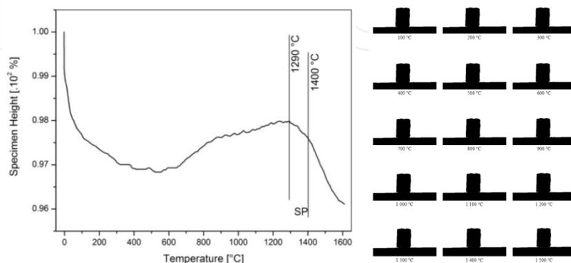
**Figure 32.** Heating microscopy of SrAC MDF specimen.
