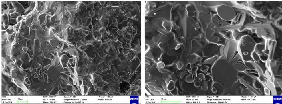
**Figure 20.** Thermal insulating refractory castables with cenospheres treated to the temperature of 1500 °C.
