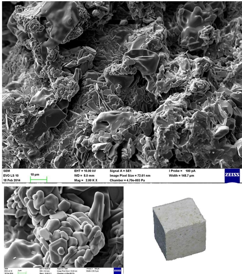
**Figure 9.** Electron microscopy image of refractory castable treated to the temperature of 1500°C.
