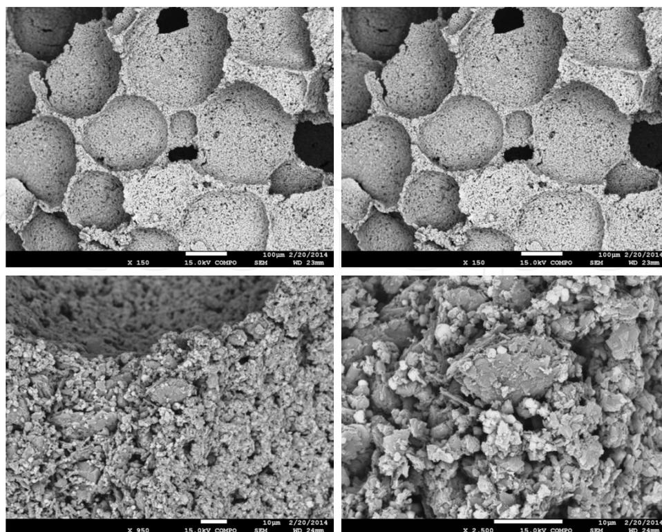
**Figure 22.** Raw foam before the thermal treatment.
