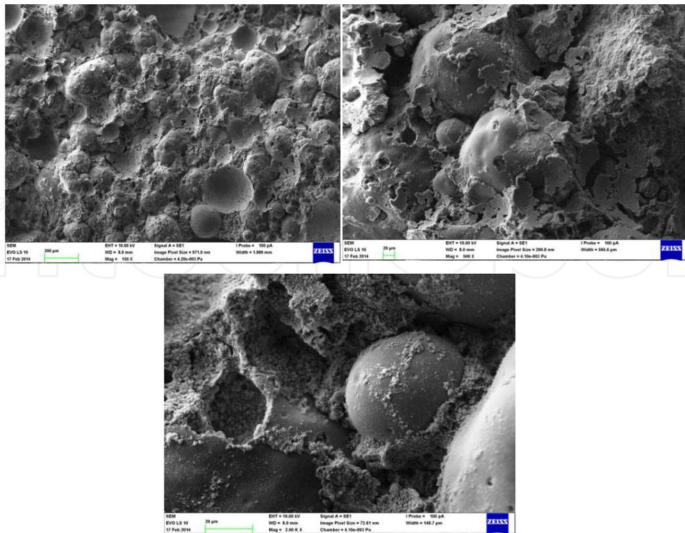
Figure 14. Thermal insulating castable based on cenospheres.
