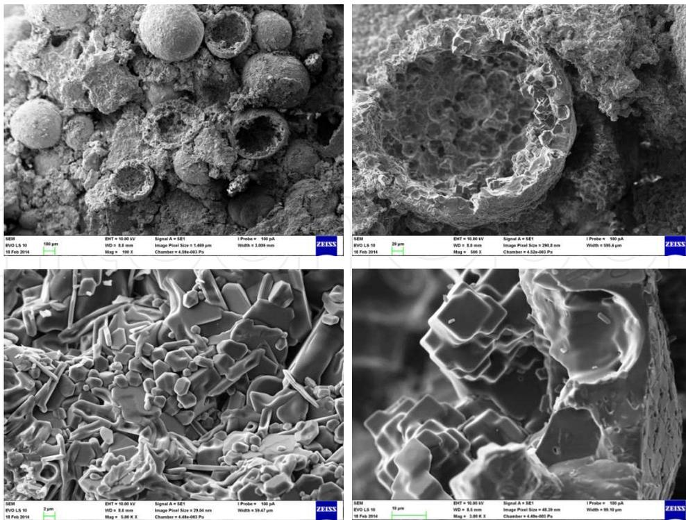
Figure 18. Thermal insulating refractory castables with bubble alumina treated to the temperature of 1500 °C.
