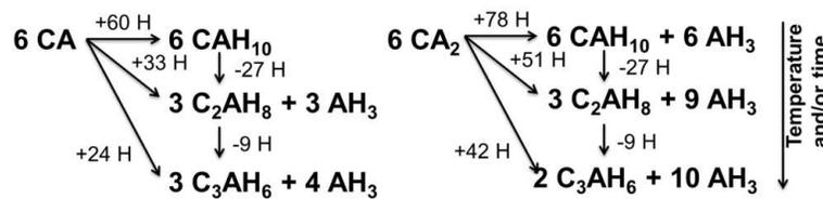
**Figure 1.** Hydration scheme of calcium aluminate cement [458].
