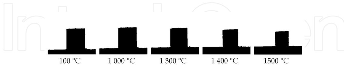
**Figure 25.** The behaviour of specimen of foam during heating to the temperature of 1550 °C at the rate of 5 °C min<sup>-1</sup>.
