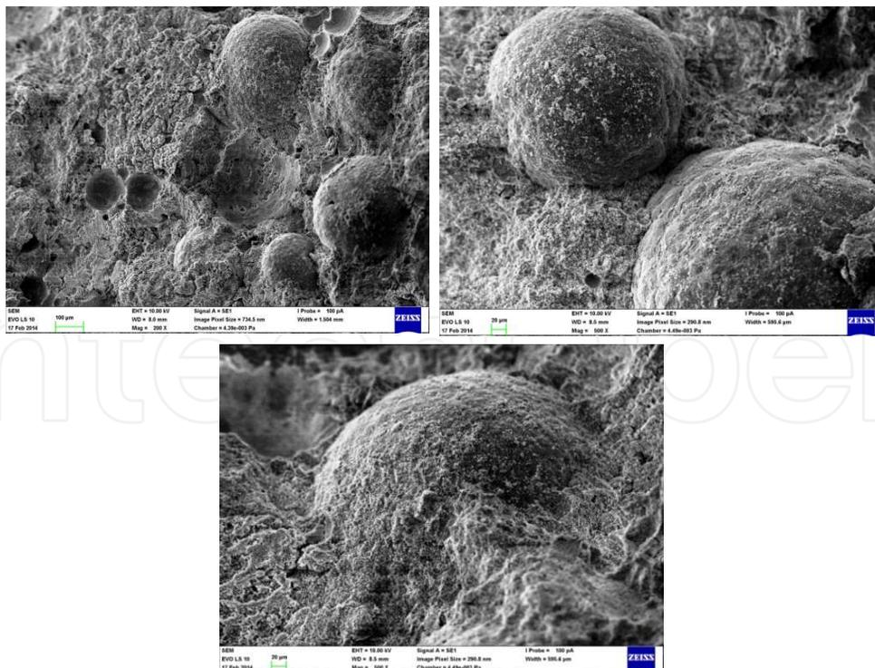
Figure 15. Thermal insulating castable filled with alumina bubbles.
