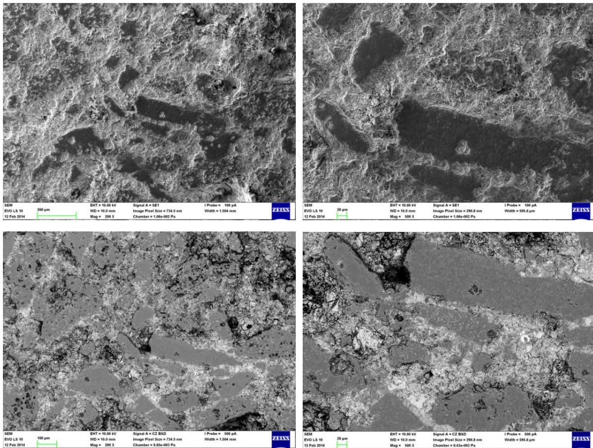
Figure 6. Electron microscopy of refractory castable before the thermal treatment.
