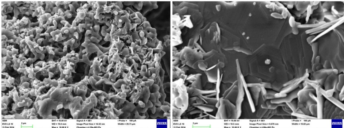
Figure 7. Electron microscopy image of refractory castable treated to the temperature of 1300°C.
