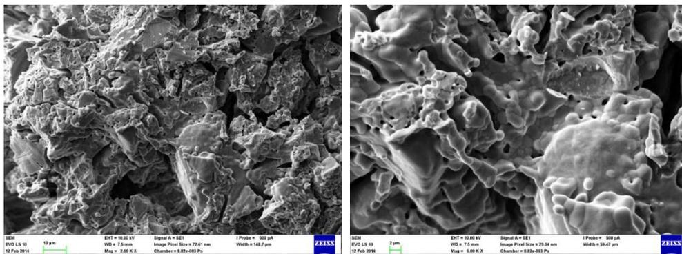
**Figure 33.** SEM image of fracture area of strontium aluminate MDF treated to the temperature of 1400 °C
