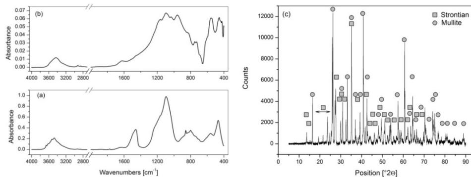
**Figure 26.** Infrared spectrum of raw foam (a), foam after the thermal treatment (b) and XRD of foam after the thermal treatment to 1500 °C (c).
