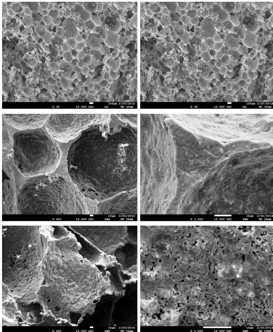
Figure 23. Foam after the thermal treatment to 1500 °C.
