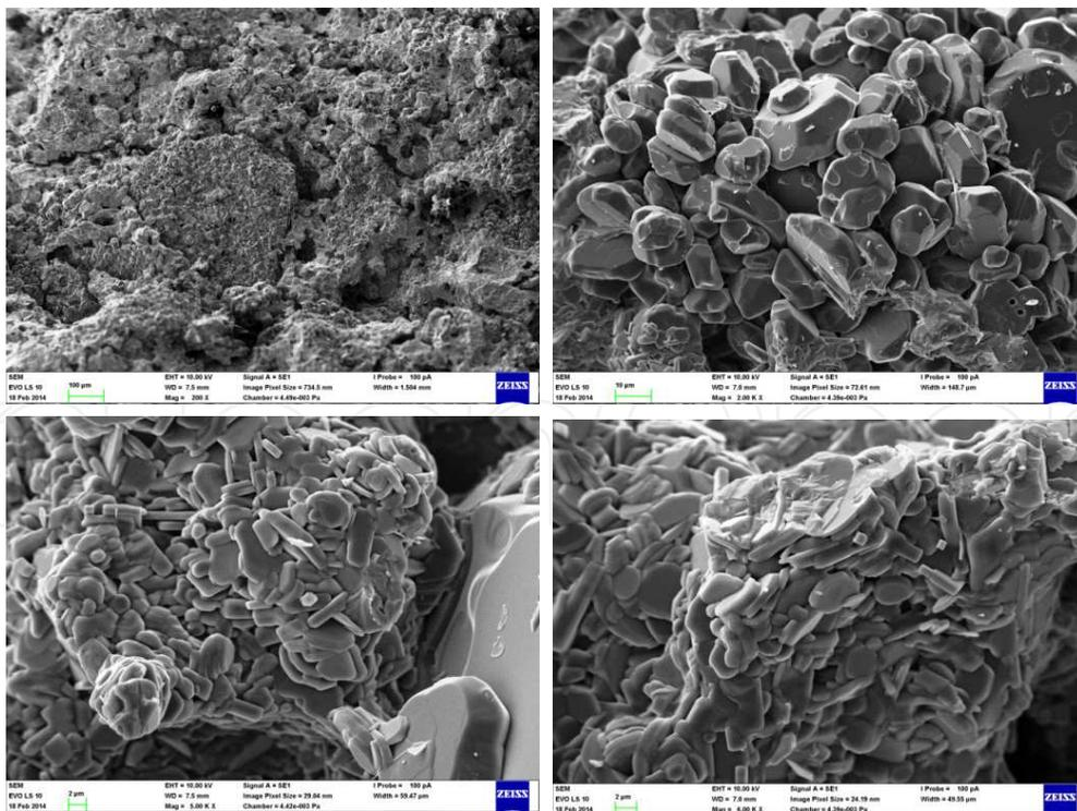
Figure 19. Thermal insulating refractory castables with fireclay treated to the temperature of 1500 °C.
