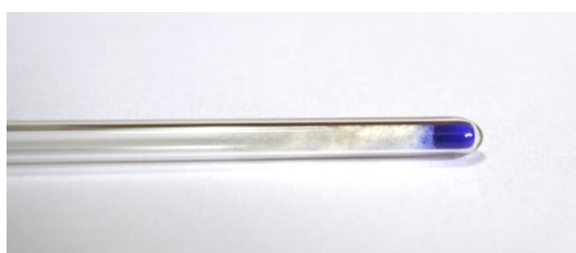
Figure 9. Ultramarine in the glass tube to EPR measurements.
