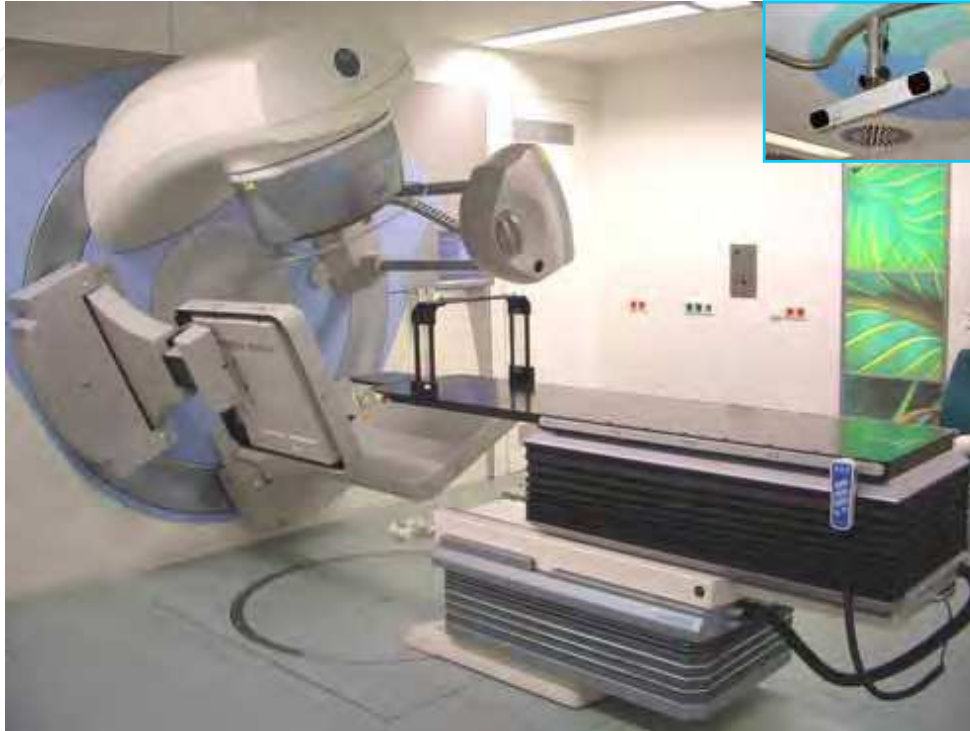
Figure 1. Linear accelerator installation at the University of Würzburg. The HexaPOD robot table is mounted on a standard treatment table. The MV treatment beam emerges through the gantry head, which in this picture is positioned at the top (ca. 340°). The MV EPID positioned opposite at the bottom (ca. 160°) records the radiation after it has passed through the patient and produces portal images. The kV X-ray source and corresponding flat panel, positioned at the right (ca. 70°) and left (250°), respectively, are rotated around the patient to produce cone-beam CT images. The inset on the top right depicts the tracking camera, which tracks the reflectors on the c-shaped bridge (see also Figure 2)
