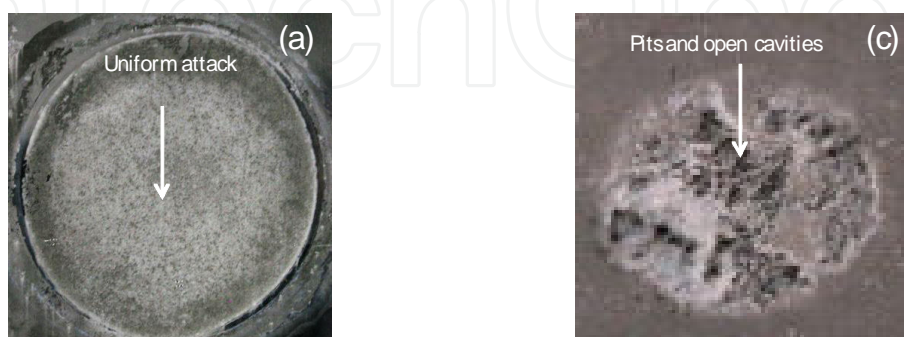
Figure 2. Surface appearance after immersion in 0.6M NaCl solution for 14 days at 24 °C and after removal of corrosion products. AZ31 specimen with the original surface in the as-received condition, Exposed circular area of ~9 cm 2 X 0.75 approx Exposed circular area of ~0.4 cm 2 X 0.75 approx
